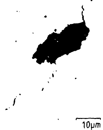
Figure 7 Closure in a crack from an inclusion
