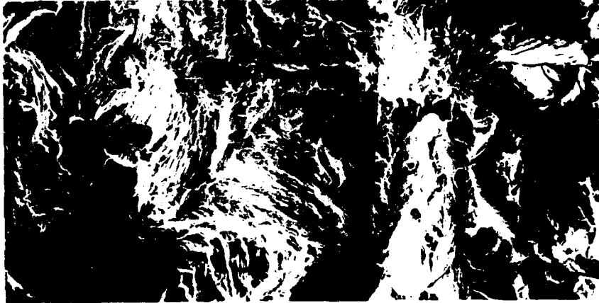
Fig. 3 The appearance of fatigue crack for pulsating waveform of load in Steel No. 1. 250X, SEM
