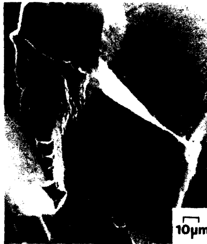
Fig. 9. Planar facets, near \Delta K_{th} , 20°C, R=0.1, prestrained 7%.
