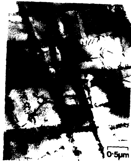
Fig. 3. Prestraining in tension. Fig. 4. Planar arrays of dislocations in specimen prestrained 7%.
