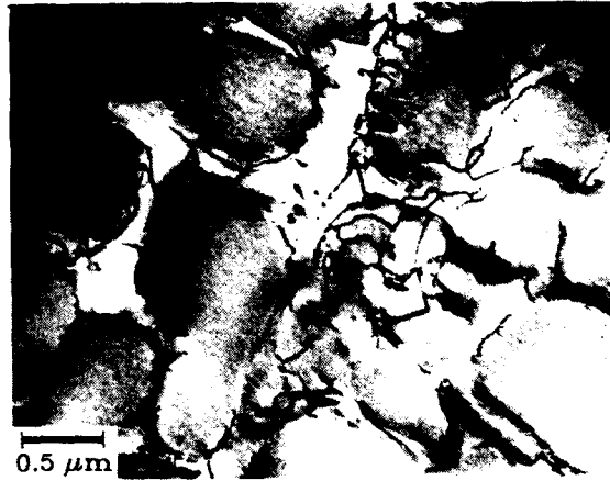
Figure 6. \gamma' by-pass at yield at high temperature. PWA 1480, 982°C, 0.3% plastic strain, 0.5%/min.
