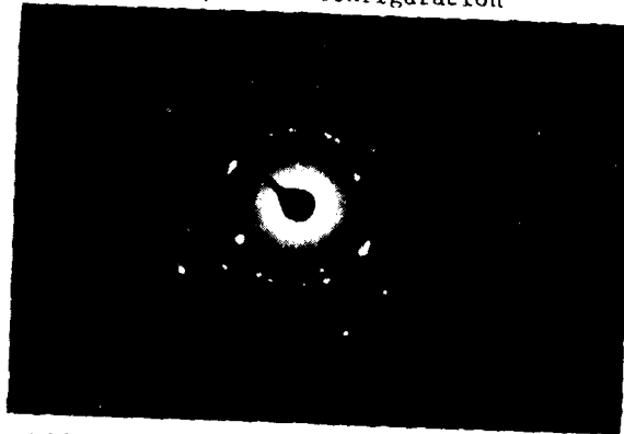
Figure 2 Diffraction pattern of Al_4C_3 formed in the interface of specimen heat treated at 545^{\circ}C
