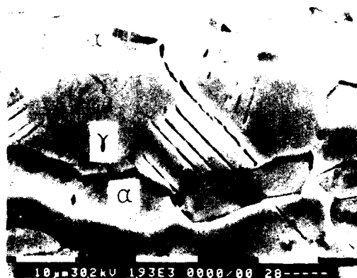
Figure 5 Corrosion fatigue crack initiation in the duplex alloy at E = E_0 , \Delta E_p/2 = 10^{-3} and \dot{\epsilon} = 10^{-2} s^{-1} .
