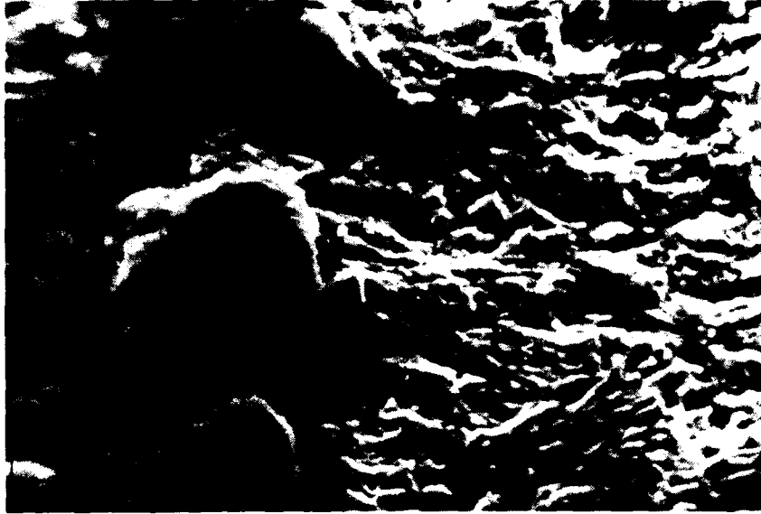
Figure 5. Nodules of oxide formed in the threshold region of a low alloy steel En 19. x 2,500
