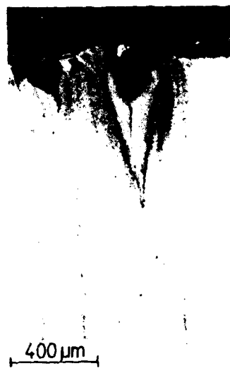
Fig.4 Metal deformation alongside the oxide wedge. A crack through the surface composite and the wedge
