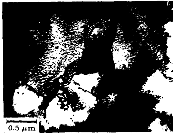
Figure 7. \gamma' by-pass and coarsening after tensile test to failure MAR-M 246, 1093°C, 0.5%/min.
