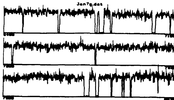
Fig. 6 Quantum jumps observed via the 280 nm fluorescence scattered from a single ^{24}\text{Mg}^+ ion held in a Penning trap. The ratio of mean "on" to "off" times for the fluorescence is observed to be 16 independent of laser intensity.
