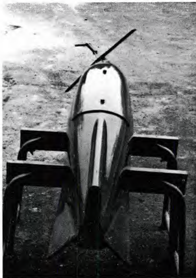
Figure 2-23. DMI Tow Body with Hydrofoil
