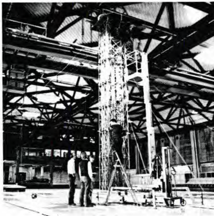
Figure 3-23. Test Set-Up of Guyed Deep Water Platform
