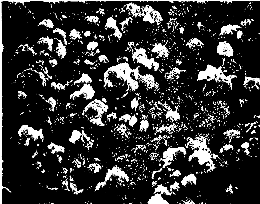
FIGURE 28. HIGH MAGNIFICATION OF AN AREA ADJACENT TO CORROSION PRODUCT BUILD-UP ON AA-6061 (2000X)
