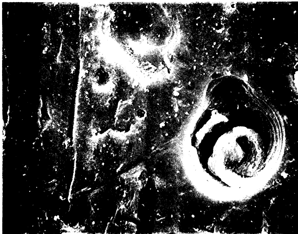
FIGURE 36 AREA ADJACENT TO A PIT ON AA 6061 (2000X)
