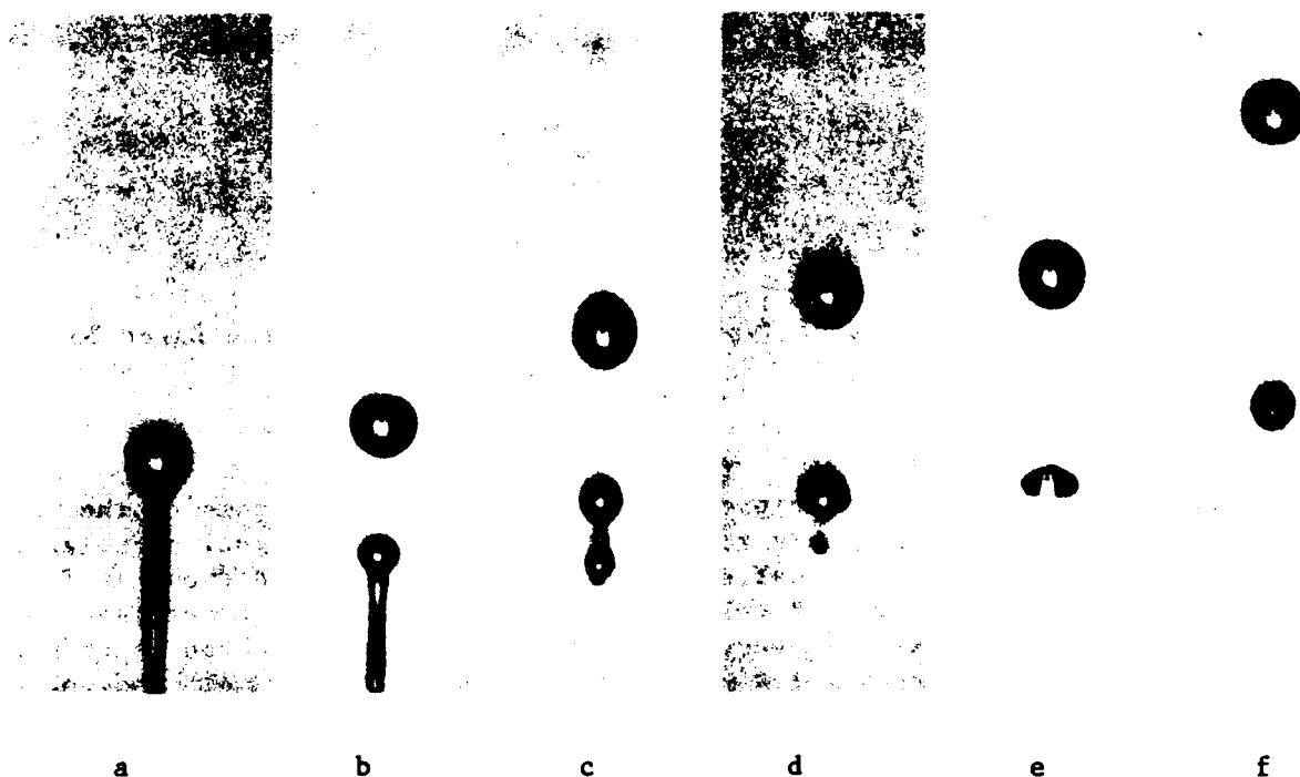
Figure 2. Complex Drop Formation Sequence. Shown are (a) drop still attached to the dropper, (b) larger drop breaking away from the dumbbell, (c-e) remaining liquid pulling together to form a smaller drop, and (f) final drops with diameters of about 270 \mu\text{m} and 200 \mu\text{m}
