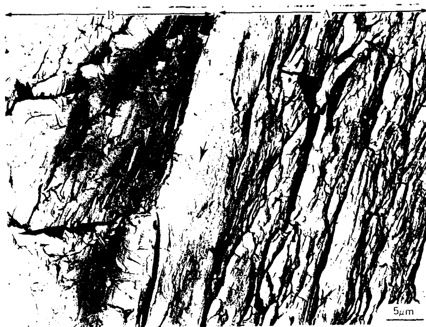
Figure 26. TEM of fracture surface produced in a magnesium crystal by rapid crack growth ( \sim 10 mm/s) in the aqueous environment, showing fluted/dimpled area (A) and cleavage-like area (B). The latter exhibits tongues associated with twins.
