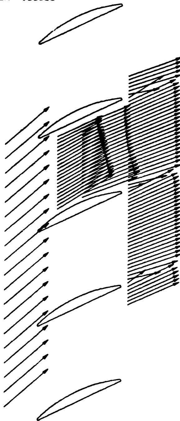
Figure 12. Measured Velocities in Blade Passage Region
