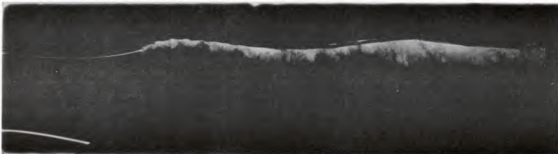
Fig. 13 — A steady breaking surface wave and the ensuing turbulent wake downstream from a submerged, towed hydrofoil. Photo courtesy of J.H. Duncan.
