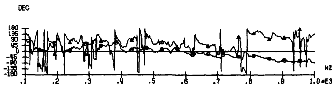
Figure 7. Comparison between Measured (1) and Calculated (2) Point Inertance in a Radial Direction in the Hull Structure with Mounted Dummy. (Vertical Scale Incorrect.)
