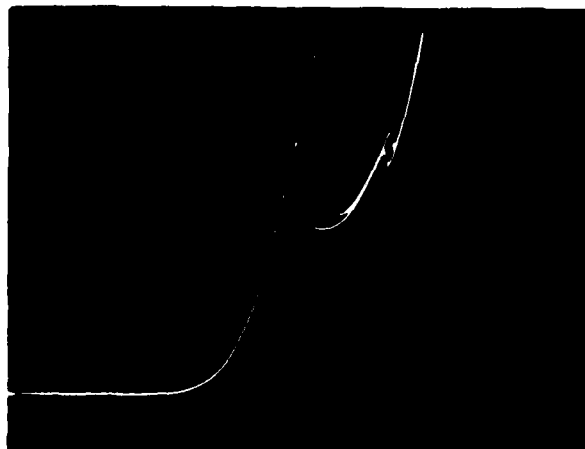
Figure 5. I-V characteristic of a 50 Å quantum well resonant tunneling device at 77°K. The higher voltage peak is due to resonant tunneling through the first excited state of the quantum well. Both of these peaks exhibited weak NDR (1 to 2%) at room temperature.
