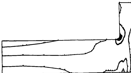
Figure 6. Plot of the maximum principal stress with concentration of stress in the corner.
