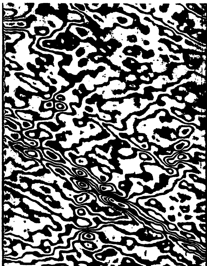
Fig. 4. Nonuniform or anomalous part of the transverse field N_x in a graphite-epoxy panel. Stacking sequence [0_2/\pm 60/0_2/\pm 60]_5 . Uniform specimen width of 25 mm (1 in.).
