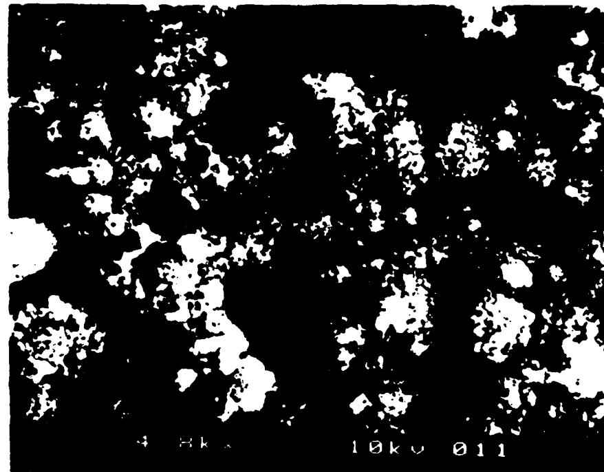
Figure 50e SEM photo -- same as Figure 50c but with greater magnification. This photo seems to indicate that the porous surface of the third level may have contained some anodization by-product.
