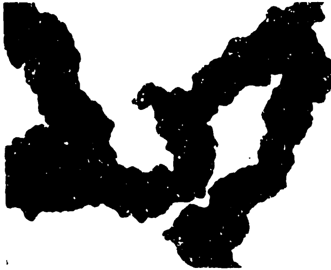
Figure 50a Dispersed dielectric breakdown observed in the third level of the MLC (200x magnification).
