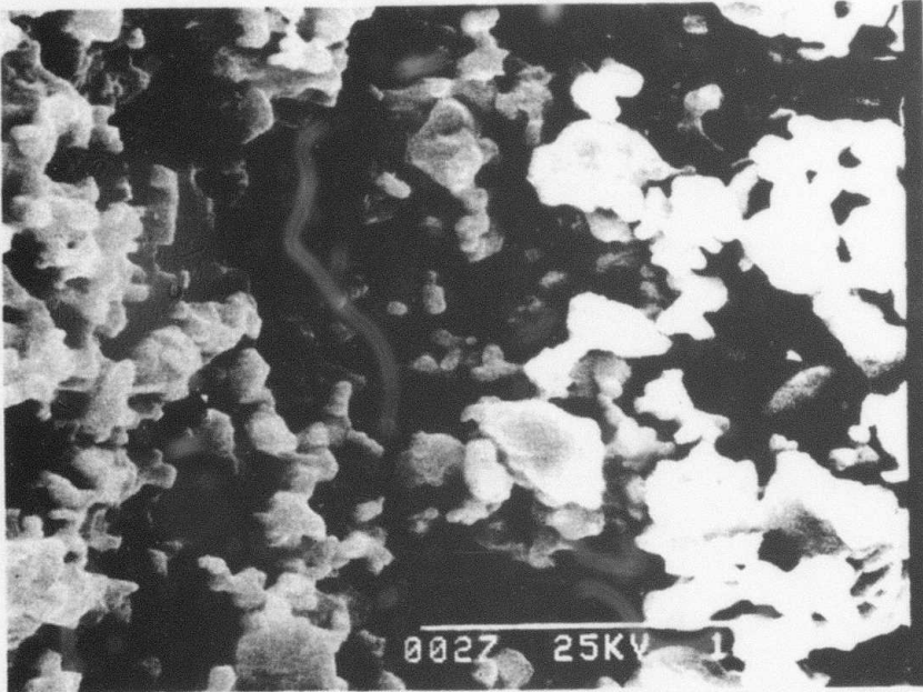
Figure 3 Primary \text{YBa}_2\text{Cu}_3\text{O}_{7-x} particles in granule after calcination at 900^\circ\text{C} 5000 X
