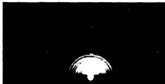
Figure 6. RHEED patterns from thin GaAs layers grown using the nucleation layer deposition and anneal steps of the three-step process.
