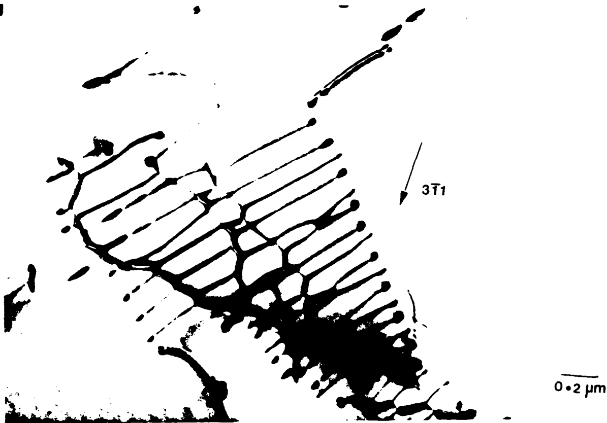
Figure 6. Electron micrograph of the intermediate stage dislocation configuration prior to recovery in In-doped GaAs deformed at 1000°C to 7.2% strain. Zone axis = [011].
