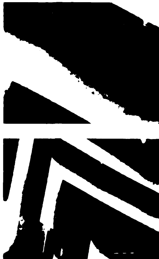
Fig. 5. Photograph of a scanning electron micrograph of a developed COP photoresist exposed as in Fig. 4. The top figure is a \times 5 enlargement of a portion of the lower panel, with the longer of the three white lines in the lower right-hand corner of the top figure being 10 \mu\text{m} in the photograph. The small spots result from imperfections in the mask and not from the lithography.
