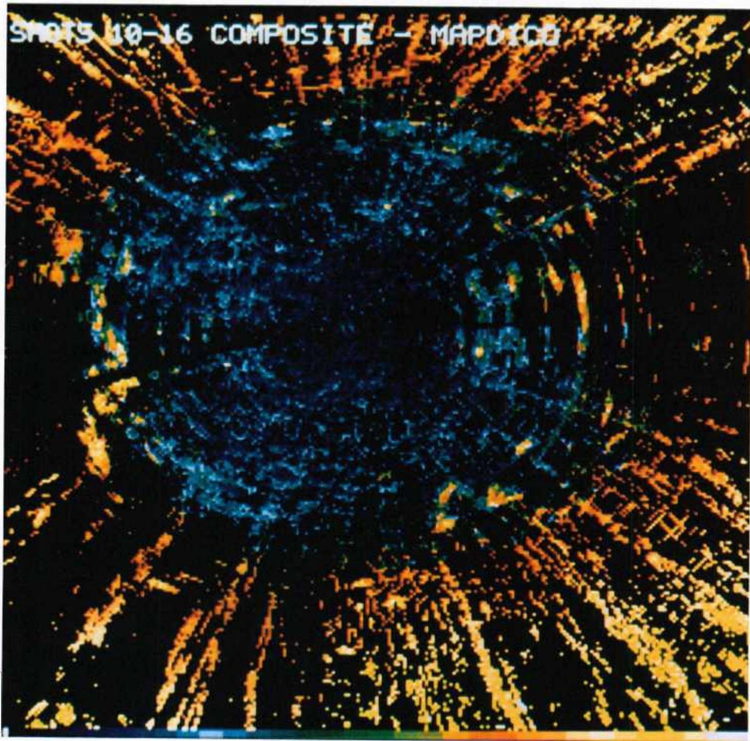
Fig. 27 — Example of integrated (averaged over shots 10 through 16) scattering strength map. Contains residual shipping noise contamination at large range from shot location.
