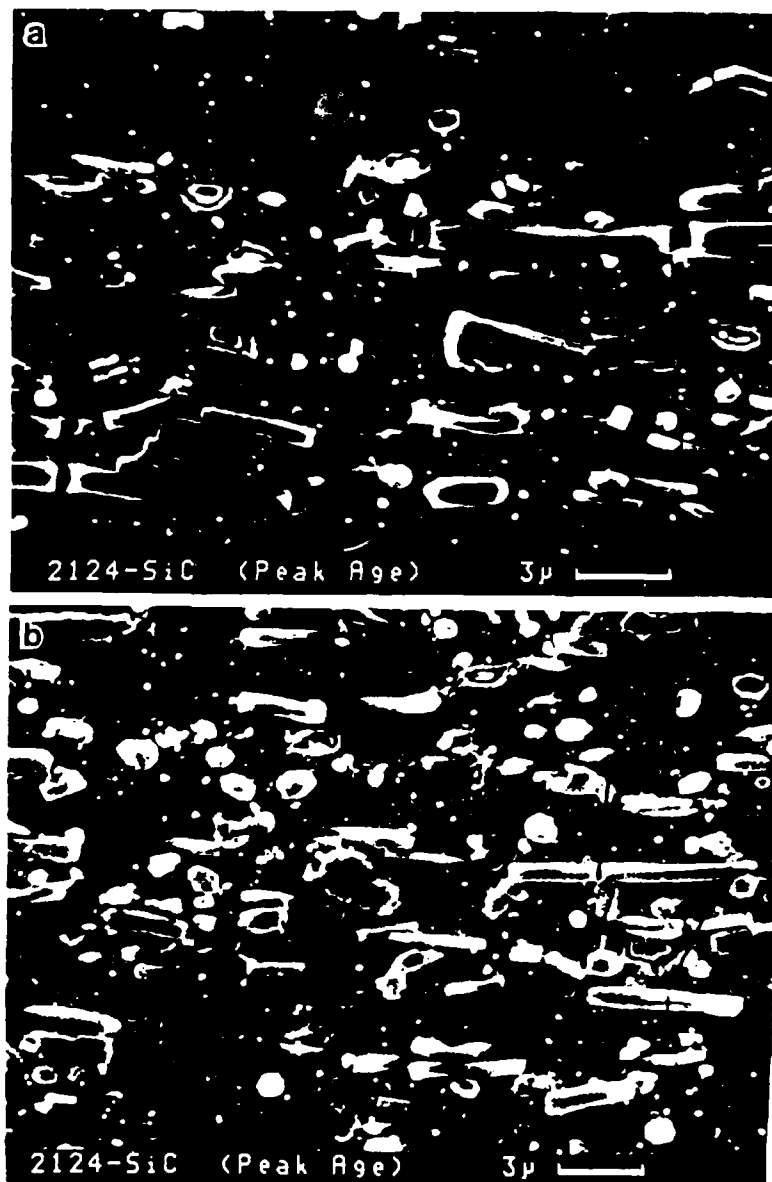
Figure 6. (a-b) SEM images of fiber cracking and decohesion (arrows) on the surfaces of SEM tensile samples
