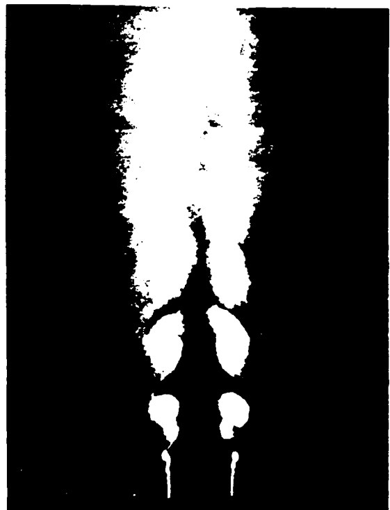
Figure 7. Axially-excited jet at Re = 50,000 ( N = 32 ).
