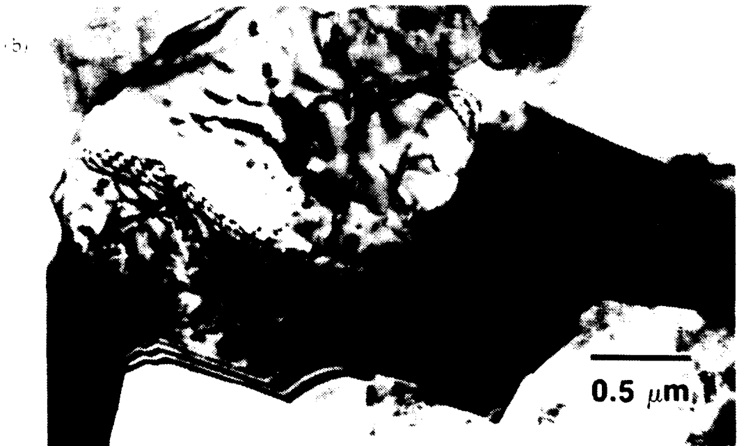
Figure 4.9 8%Mg-1%Li Aged at 120°C for 168 Hours, Recovered Region
