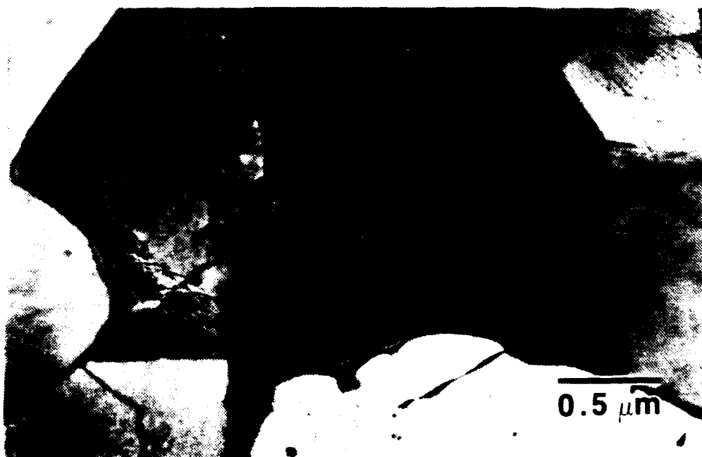
Figure 4.20 6% \text{Mg} -2% \text{Li} Annealed, Recovered Region
