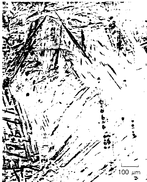
FIGURE 2 MICROSTRUCTURE OF Du-3/4 Ti ALLOY (Polarized Light)
