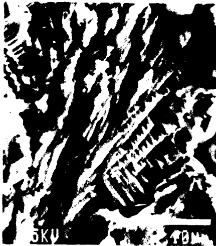
Figure 6 Near-threshold facet for 70-30 \alpha -brass in air, with two regions of striations separated by more complex region
