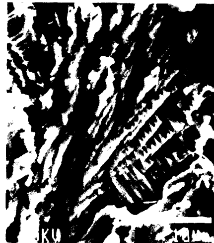
Figure 6 Near-threshold facet for 70-30 \alpha -brass in air, with two regions of striations separated by more complex region
