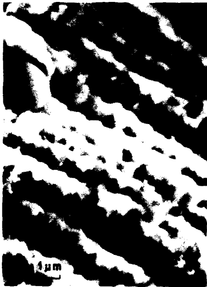
Figure 7 Striated threshold facet for copper tested in air
