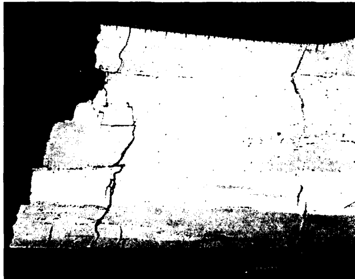
Figure 2 HTLCF specimen tested under strain wave with hold time in tension showing multiple cracking
