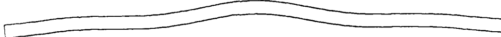
Figure 43. Buckle deformation shapes from DYNA2D with 2100 taps, h = 0.635 mm, D = 26 mm, S_r = 2.4 .
