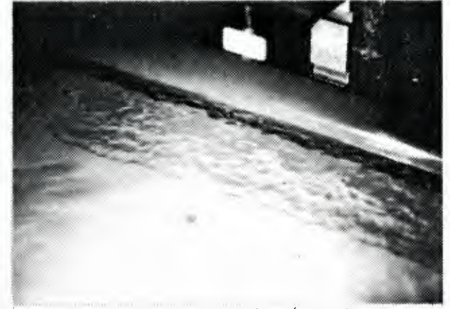
1c- Velocity \sim 55 cm/sec (fully turbulent).
