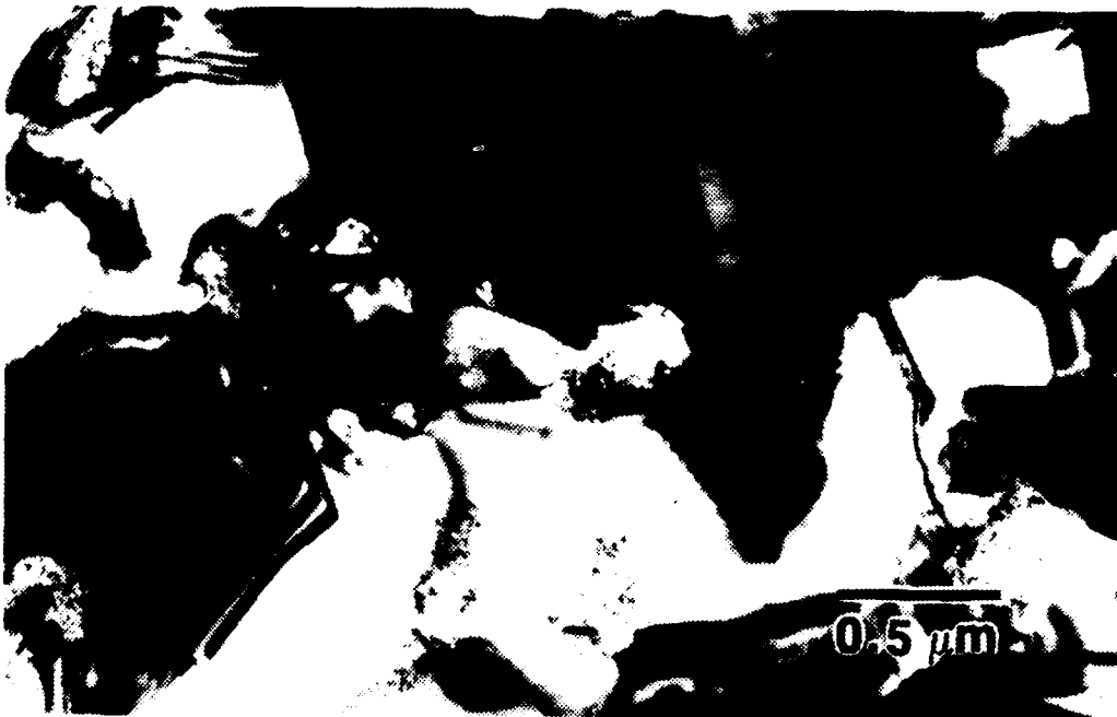
Figure 4.24 6-2 following 1 hour anneal at 300°C
