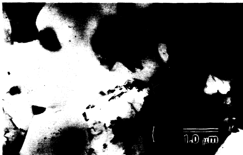
Figure 4.19 6-1 following deformation at 1.7 \times 10^{-2} \text{ sec}^{-1}
