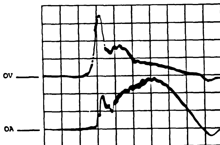
Figure 2-4. Typical Control Grid Voltage and Current
