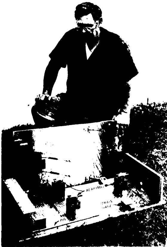
Figure 5. Instrumented section for measuring sliding and uplift forces
