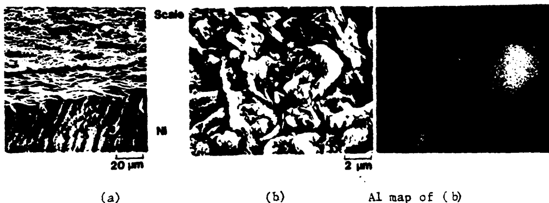
Figure 8. Nickel exposed for 30 min. at 710^\circ\text{C} at 18^\circ impact angle to 190\text{ ms}^{-1} airflow. (a) Removal of scale from metal facilitated by electropolishing in \text{H}_2\text{SO}_4\text{-H}_2\text{O} bath at 1.5 volts for 20 minutes. (b) View of underside of stripped scale showing embedded \text{Al}_2\text{O}_3 particles.
