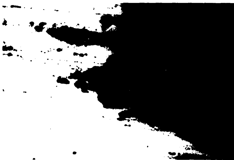
Figure 63. Severe pitting in surface of C-ring after Test VI exposure (200X)
