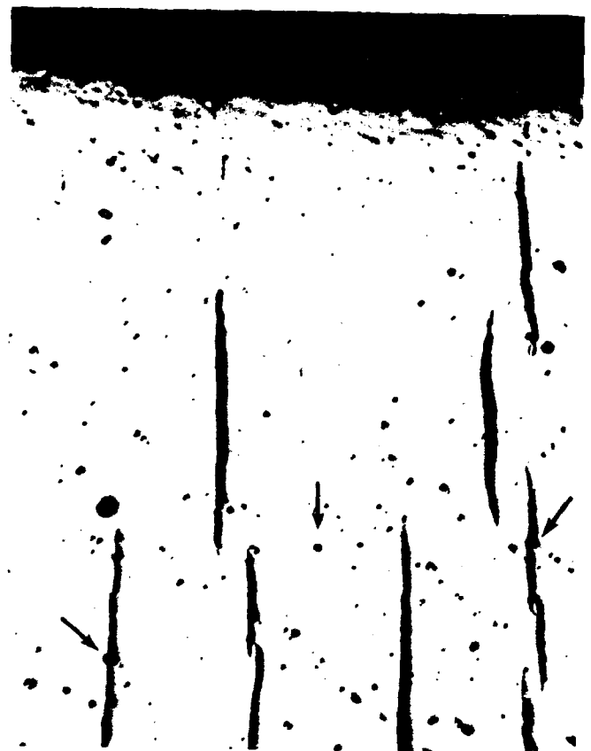
Figure 16. Longitudinal section reveals inclusions within the material, Mag. 500X.
