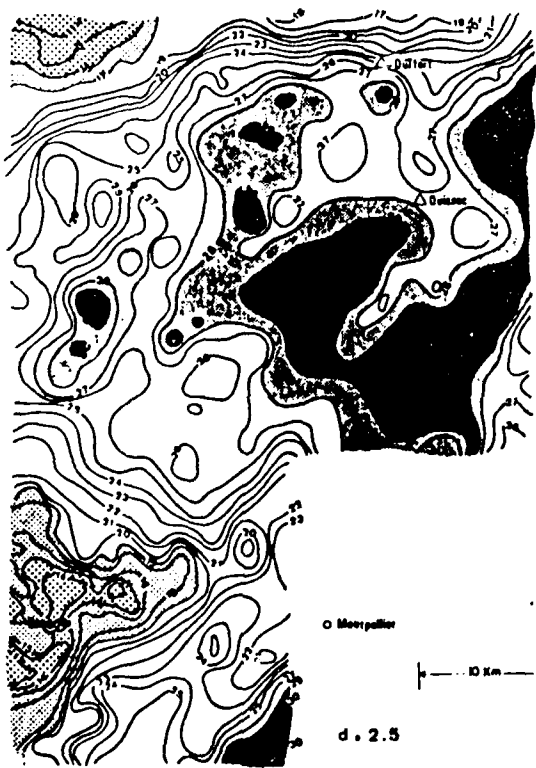
Fig. 5. Isostasy-corrected Bouguer anomaly map, for a constant 2.5 \text{ g cm}^{-3} density, including old stations only (values in milligals).
