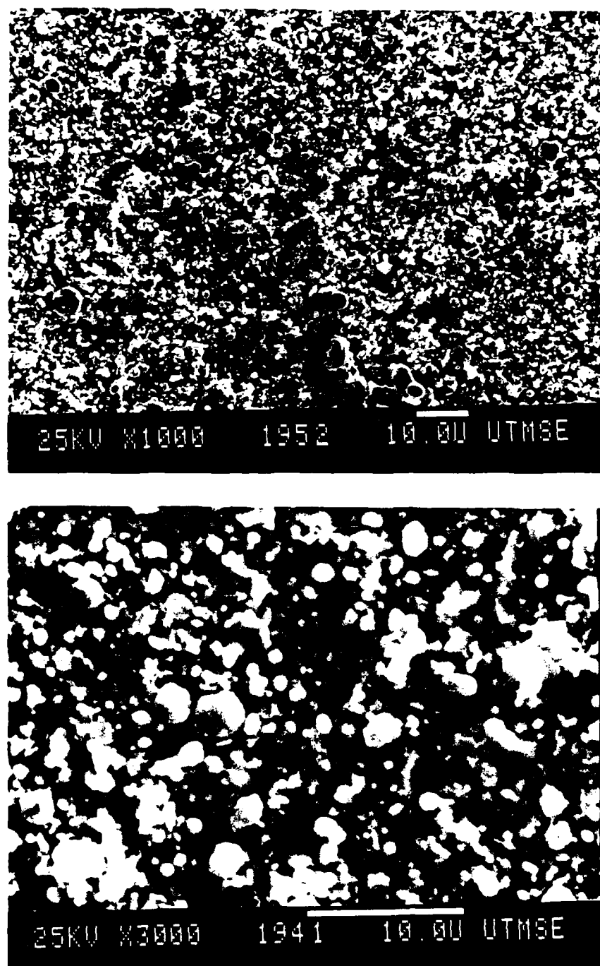
Figure 13: SEM Micrographs of Shot # 195 Co-deposited Al and Mo, Notice the much smaller liquid droplet size ( \approx 5 \mu\text{m} down) and lack of surface splatting effect. a) Low Mag., b) High Mag.
