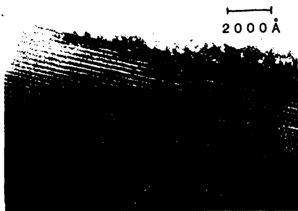
FIG. 2. Cross-sectional TEM image (bright field). Coherently strained and dislocation-free layered structures (200-Å period) have been observed.
