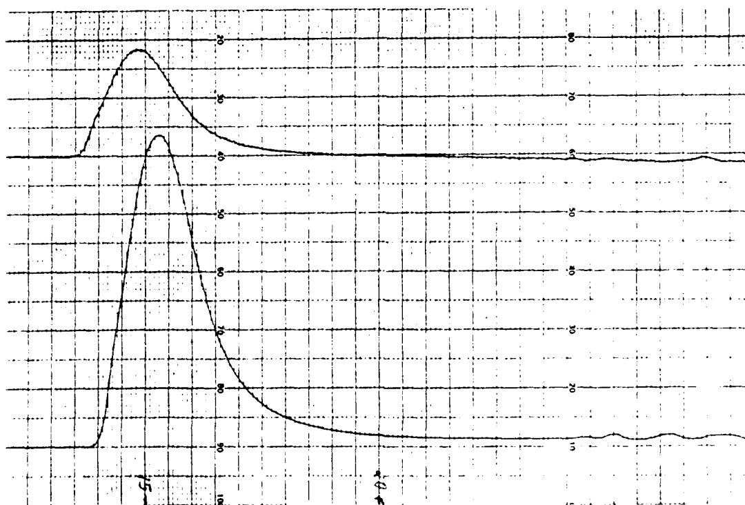
Fig. 42. GP Chromatogram of FPF-1 ( M_n = 2100 ) Chain-extended with 3,3-Dinitropentane Diisocyanate
