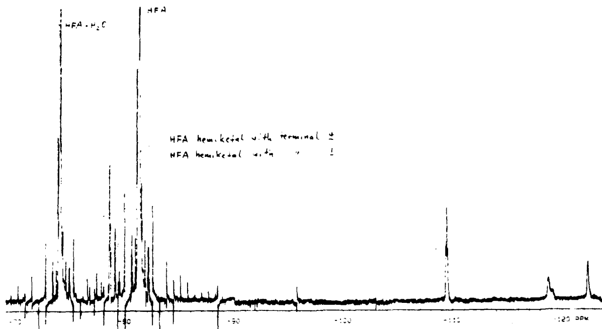
Fig. 10. ^{19}\text{F} -NMR Spectrum of a Copolyformal of 5 and 8 (15:85, 20g Sample) after addition of hexafluoroacetone.
