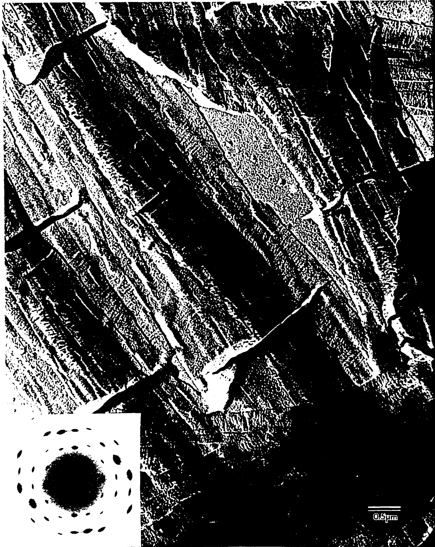
Figure 7 Electron micrograph of solution grown PBPP crystals with its electron diffraction pattern insert.
