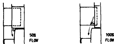
(B) MOVING SIDEWALLS.
