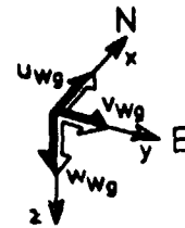
Fig. 6: Definition of Wind Components
