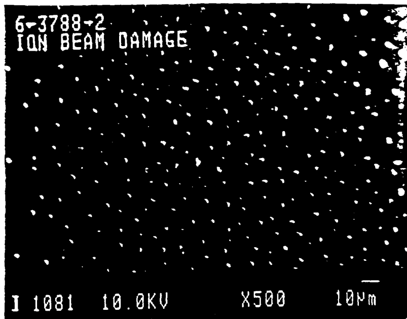
Figure 5. Damage blisters which resulted from 12.5 minutes ion beam sputtering at 2 KeV. The ion beam current density was at least 2 orders of magnitude lower than the electron beam current density used in Figure 2.
