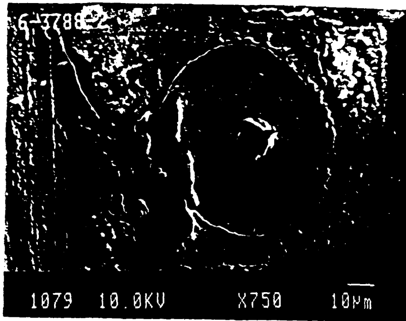
Figure 3. Electron beam damage at crater #1. A 10 KeV electron beam at 2 microamps was rastered over a 125 micron by 88 micron region. Melting, blistering, and cracking damage is apparent.
