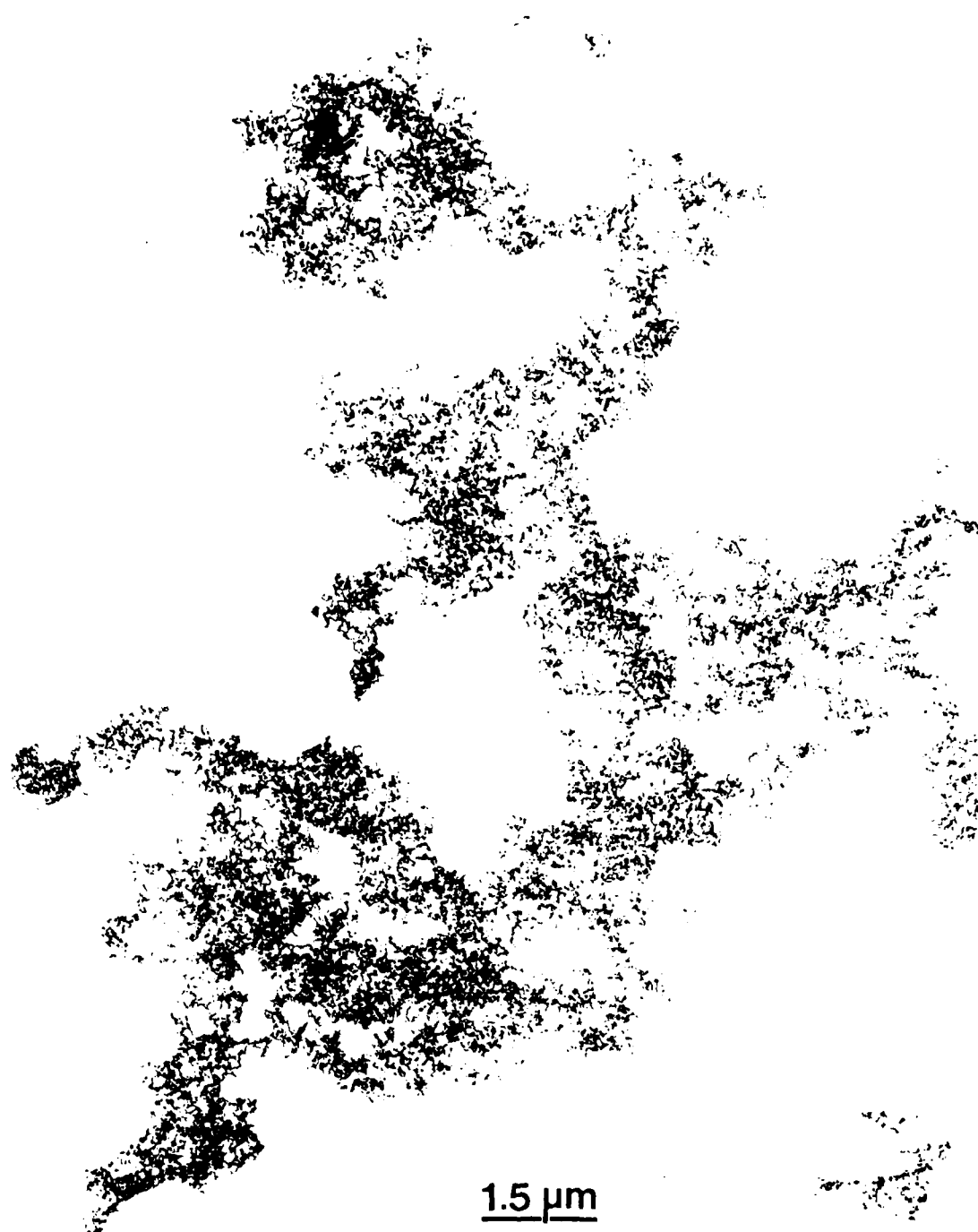
Fig. 7. A transmission electron microscopy image of a cluster of gold particles (diameter 15 nm). The cluster is a fractal object; the fractal dimension can be determined by a
