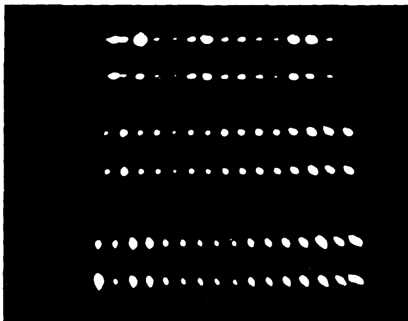
Figure 1-4. Near-field pattern of a hybrid two-dimensional surface-emitting laser array consisting of three 4\text{-mm} -wide GaAs/AlGaAs linear bar arrays mounted in three separate grooves on a common Si substrate.
