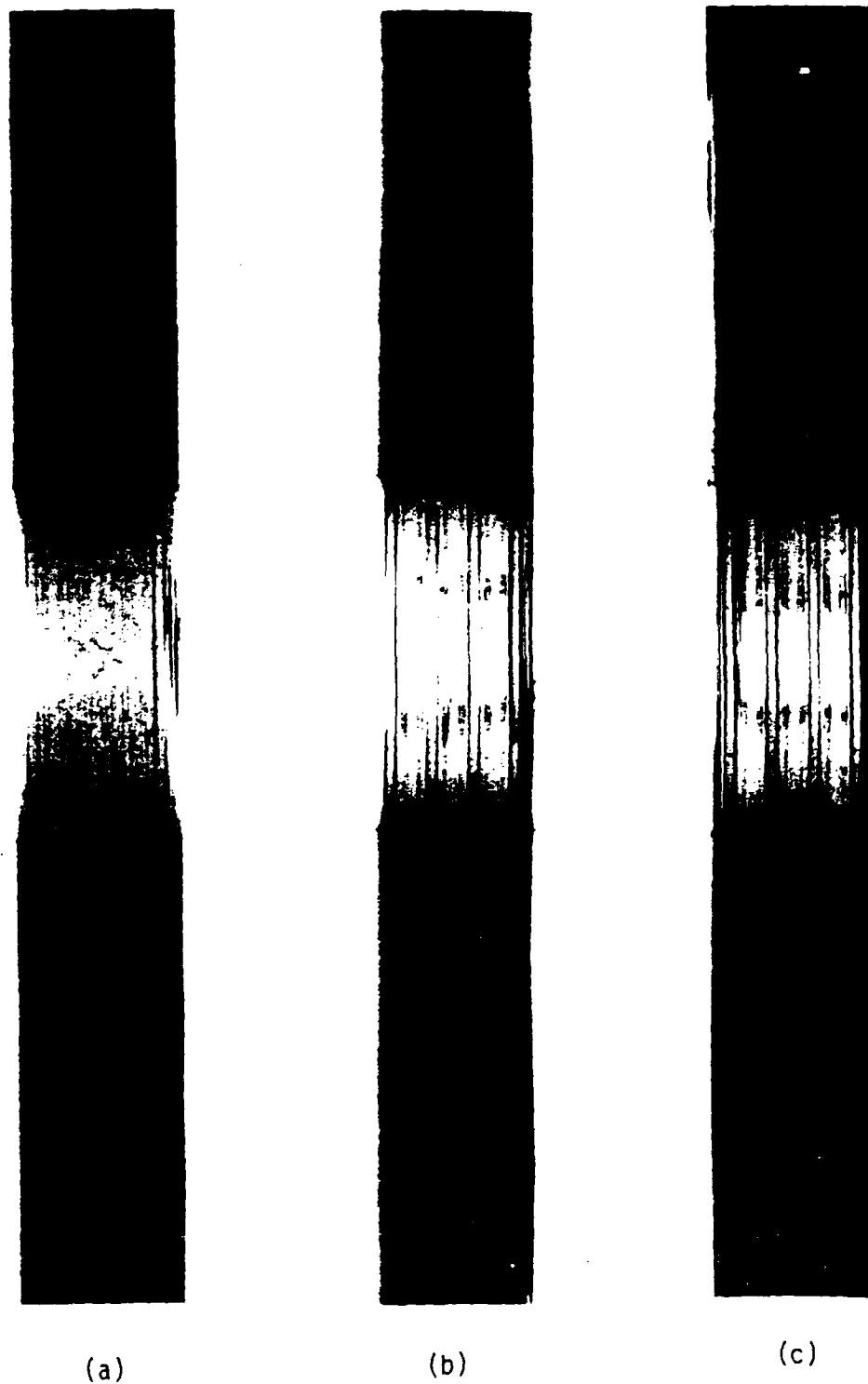
Figure 47. Edge radiographs of center-notched, AS4/1808, (0,45,0,-45)_{34} specimens during high-load fatigue: (a) early; (b) middle; and (c) late life
