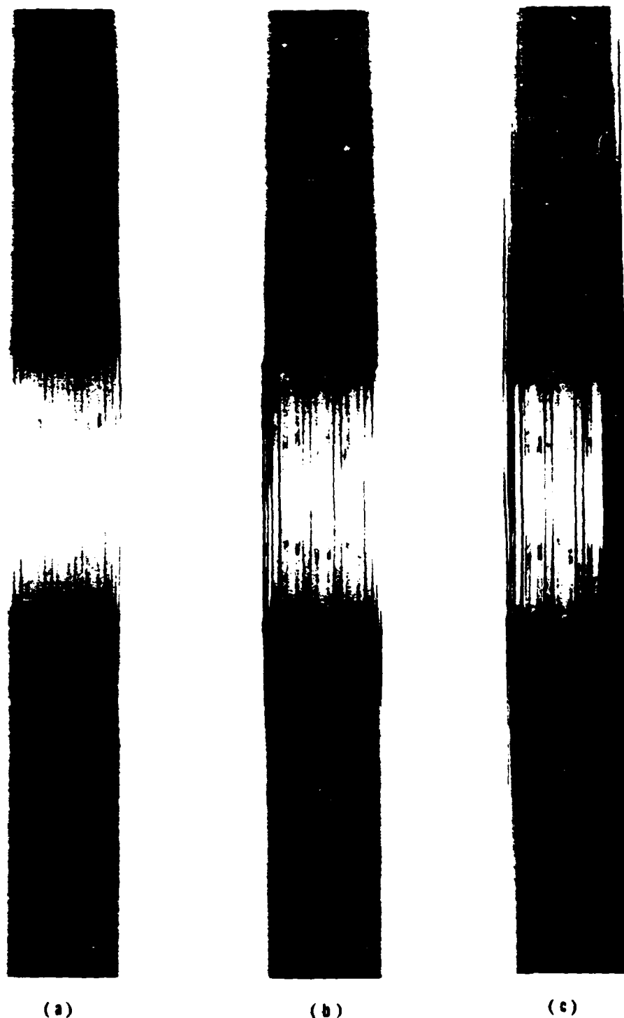
Figure 32. Edge radiographs of center-notched, AS4/3501-6, (0,45,0,-45) s4 specimens during high-load fatigue: (a) early; (b) middle; and (c) late life
