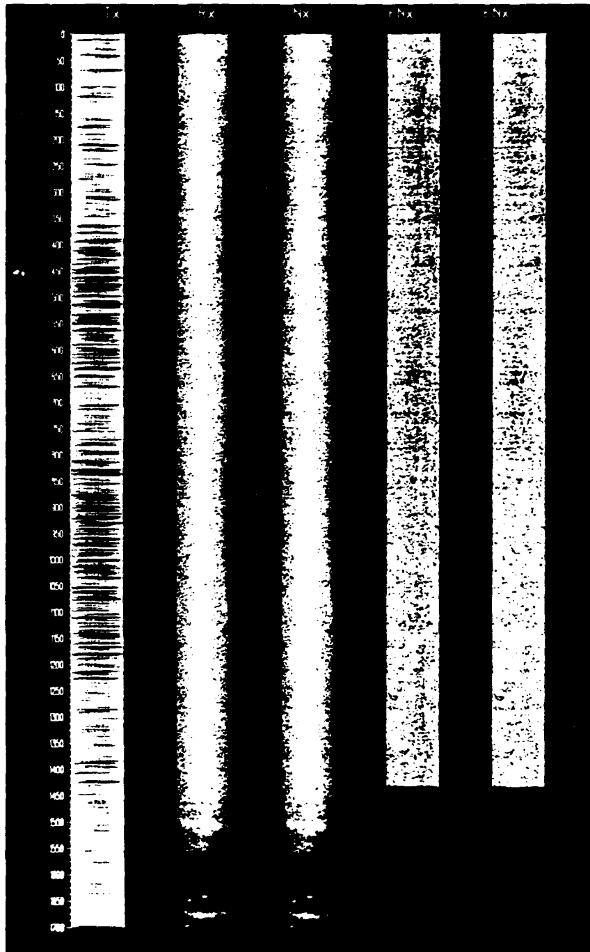
Figure 11. OSRMS image showing the wake of the freighter FRUITION. Taken on 1987 Aug 19, 12:28 to 12:31, at 48^{\circ}45'N , 126^{\circ}45'W . The wind is 5 m/s towards 090^{\circ}T and the freighter's speed is 7 m/s.
