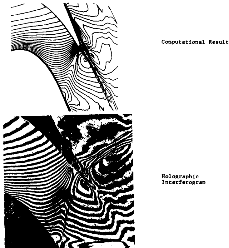
Figure 3.29 Holographic interferometry of transonic flow in cascades.
