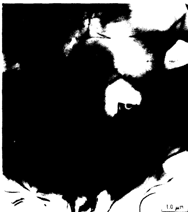
FIGURE 7. TEM MICROSTRUCTURE OF 30 MOLE % AlN ALON MATERIAL; SAME MATERIAL AS IN FIGURE 6(c).
