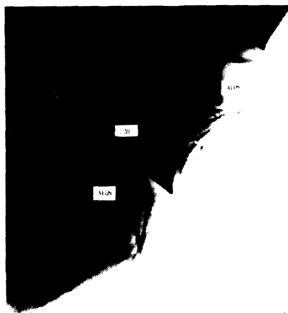
FIGURE 12. TEM MICROSTRUCTURE OF 12H PHASE IN ALON MATRIX; SAME MATERIAL AS IN FIGURE 10(c).
