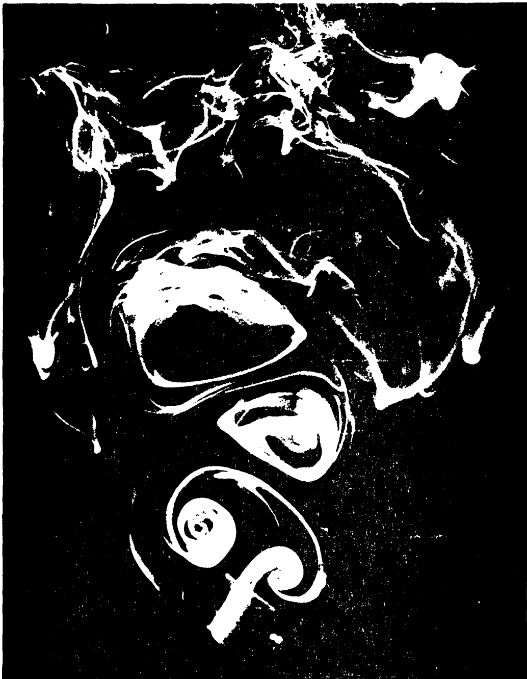
Fig. 10 Single photograph of well-tuned mode 2 hover-jet. h_a/c = 1 , \alpha_a = 33^\circ , f = 1.3 Hz, R_f = 300 .
