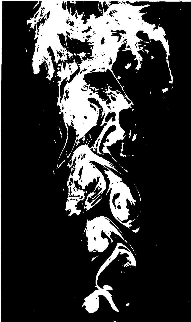
Fig. 3 Single photograph of a hover-jet for mode 1 hovering of the airfoil. h_a = 2.54\text{cm} , \alpha_a = 68^\circ , f = 1\text{ Hz} , h_a/c = 1 , R_f = 230 .
