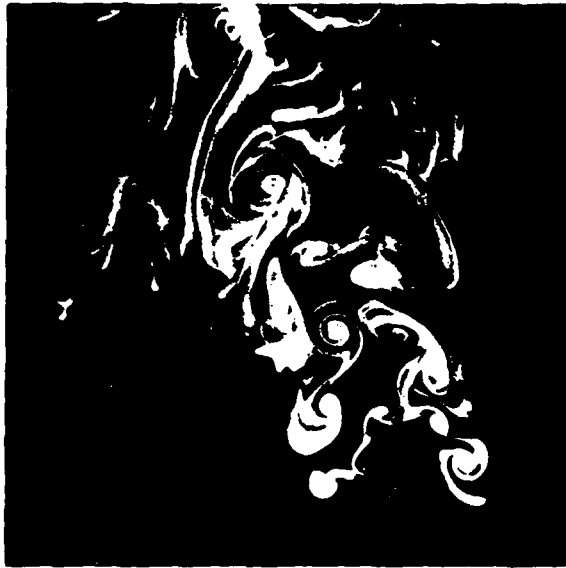
Fig. 11 Single photograph of mode 1 hover-jet far from optimum thrust. h_a/c = 1.5 , \alpha_a = 25^\circ , f = 1 Hz, R_f = 340 .
