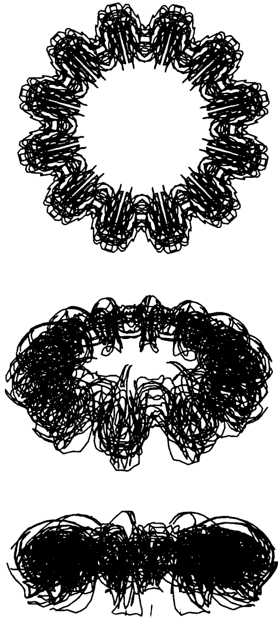
Figure 6. Three perspective views of the vortex ring shown in Fig. 4 taken at t = 140 . \phi = 0^\circ, 60^\circ and 90^\circ . The ring propagates upwards (and out of the page.)
