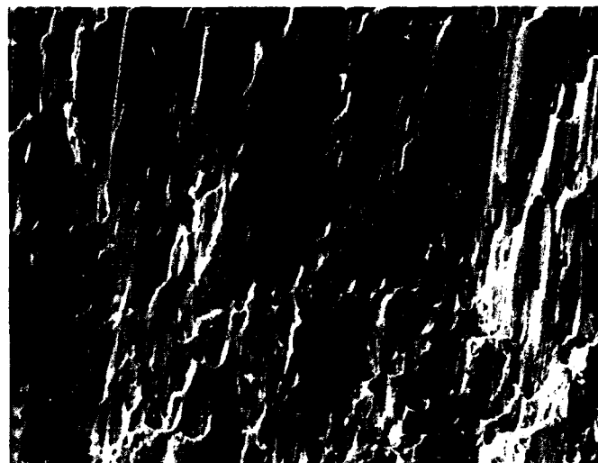
Figure 1: SEM Micrographs of Chips of Free-machining Brass (Workpiece Speed 100 m/min) left: Rough side of chip right: Smooth side of chip
