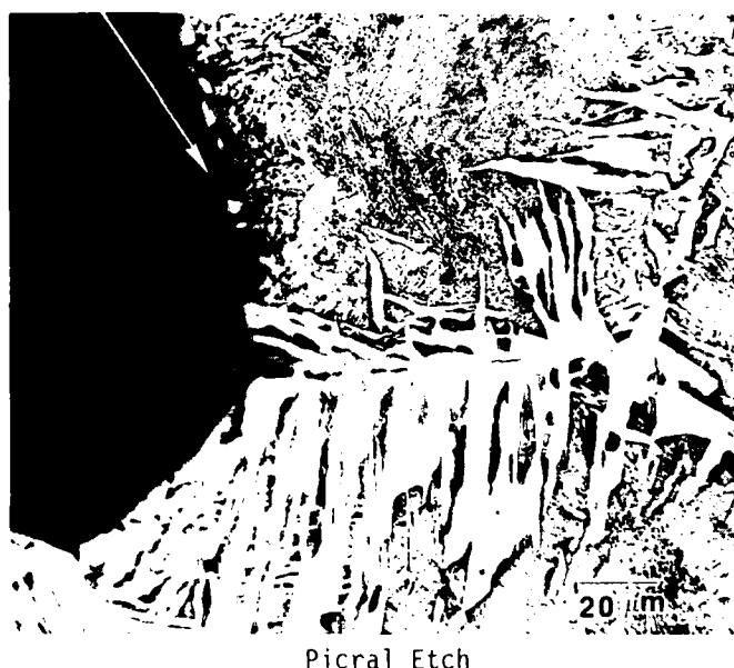
Fig. 6 - Intergranular fracture along prior austenite grain boundaries in a field failure
