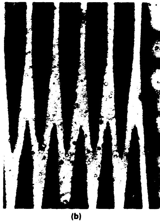
Figure 1-7. Y-junction-coupled laser array: (a) schematic illustration, and (b) top view of a portion of an IBAE-defined mesa.
